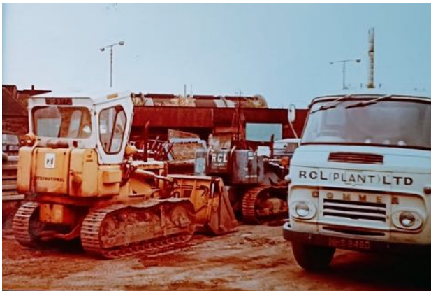
Figure 5: 1980: The International drotts used for 'can crushing' at Fountain (better camera by now).
