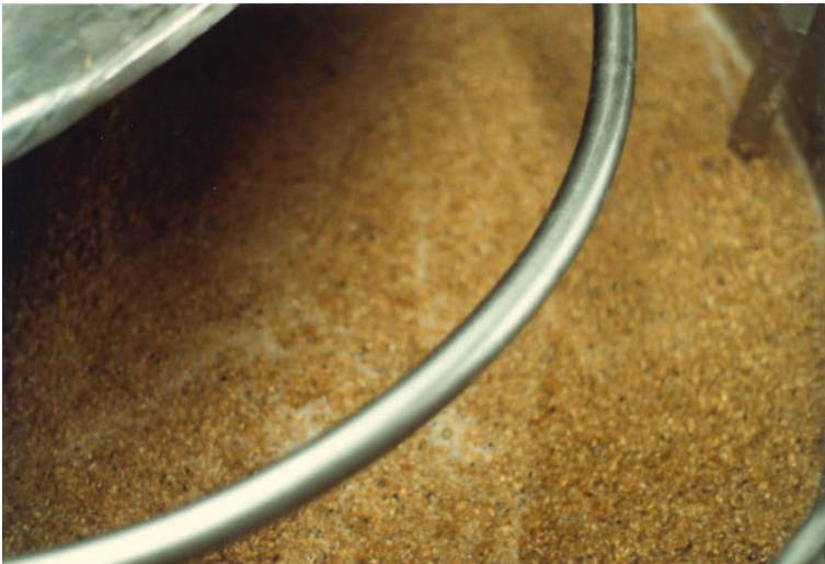
Figure 4: After mashing, the hose-tail with the incoming water was replaced with the sparge ring which had holes in the underside, enabling the sparge to be added after first worts were run off.
