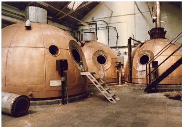
Figure 8: After the wort is transferred from the lauter tun to the copper or sometimes called the wort kettle, it is brought up to boiling point. Thereafter hops are added to give bitterness, flavour and aroma to the wort. Holyrood had five coppers, each containing 100 barrels, equivalent to 28,800 pints.
