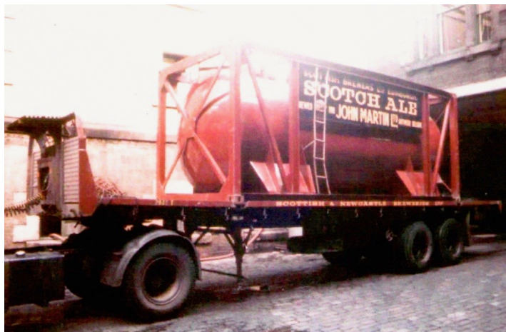
Figure 1: A 90-barrel tank demountable of Scotch Ale (No. 3 Br.) destined for John Martin Ltd in Belgium.
