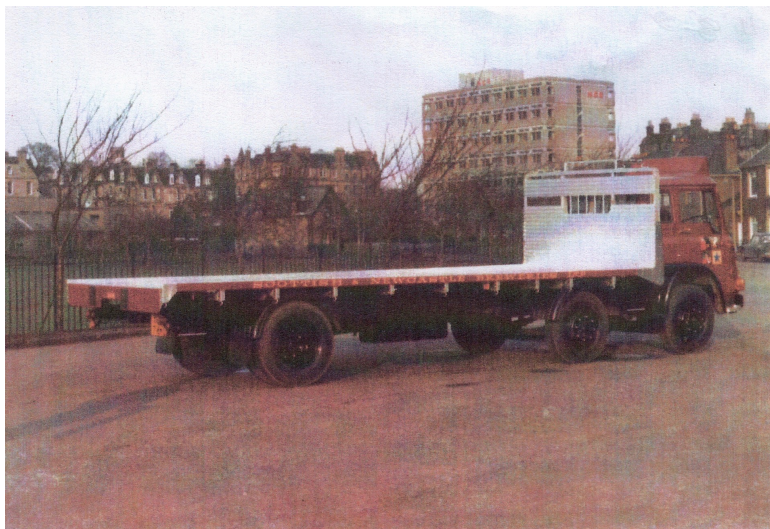
Figure 13: A publicity shot of a large capacity dray seen at Roseburn Park adjacent to SMT Commercial's Edinburgh premises where many hundreds were built for S&N. It is a Bedford KG twin-steer three-axle 14.5 ton flatbed with a nine ton payload.
