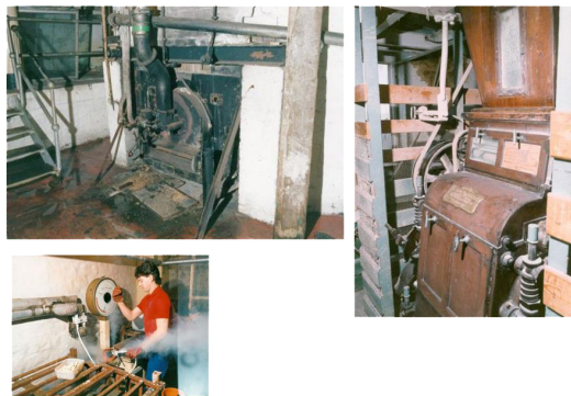
Figure 7: Top left: The “copper fire” – heavy fuel oil fired. Right: Seck mill. Below: Filling CO 2 cylinders.
